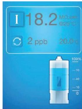
► **Type I water output** from the Cascada II.I system meets or exceeds Type I water standards as specified by ASTM, CAP, ISO 3696, CLSI, JIS K0557 and high-purity water as described in USP, EP and ChP. Type I water is required for critical laboratory applications such as:
