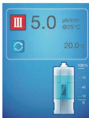
► **Type III water** is required for sensitive laboratory applications:
