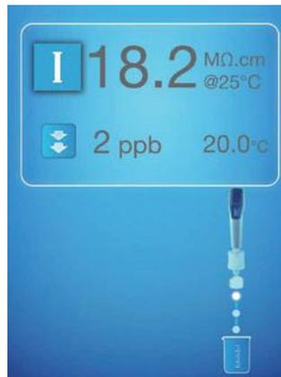
► **Type I water output** from the Cascade III.I system meets or exceeds Type I water standards as specified by ASTM, CAP, ISO 3696, CLSI, JIS K0557 and high-purity water as described in USP, EP and ChP.
